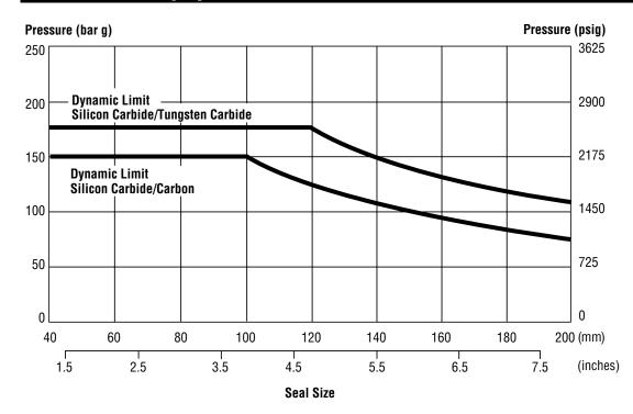
The basic pressure rating is for a standard seal, as shown in the typical arrangement, when installed according to the criteria given in this data sheet and generally accepted industrial practices.
