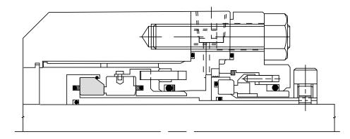
The dry tandem arrangement uses the high duty version of the SBOP backup seal to provide operational security without the expense of a liquid buffer system. In the event of failure of the inner seal, the SBOP will prevent loss of the pumped fluid to the atmosphere. This can be detected by use of a pressure switch.
