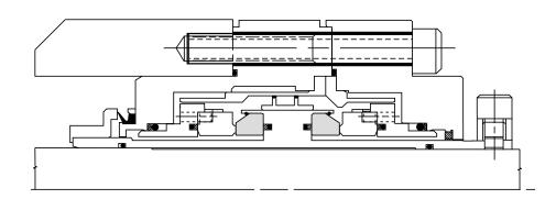
This dual pressurized (double) arrangement consists of two seals face to face and operating on a barrier liquid. Any leakage from the inner seal will be of barrier fluid into the pumped product. The inner seal includes a double balance line for reverse pressure protection.
