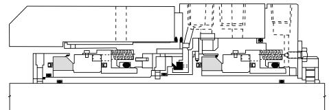
The dual, unpressurized (tandem) arrangement consists of two seals in series. The inner seal operates on pumped fluid and the outer seal normally operates on a low pressure buffer liquid. The outer seal is designed to provide a full-duty backup service.
