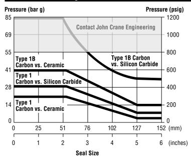
To determine the maximum pressure for the Type 1 or 1B required, multiply the maximum pressure by the multiplier factors to obtain the maximum operating pressure.
