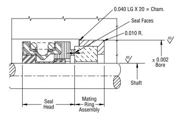
See the seal layout and the Type-6 bulletin for critical dimensional and tolerance data before starting assembly.
