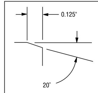
**NOTE:** If the measured dimensions exceed the values given, correct the equipment to meet the specifications before installing the seal. If the seal is installed on a sleeve, the sleeve must be liquid- and pressure-tight through its bore. The thickness of the gland plate must be sufficient to retain the service pressure without distortion.
