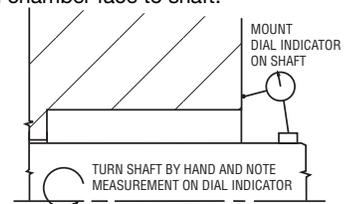
4. Measure shaft runout (with respect to seal chamber - see above table).
